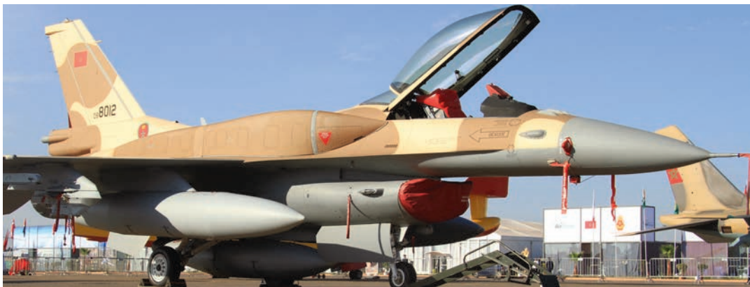
A RMAF F-16C 08-8012 fitted with conformal fuel tanks can operate the Sniper targeting pod and DB-110 reconnaissance system. The aircraft are useful assets in the Saudi-led coalition in Yemen.
