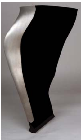
The LEAP-X (top) and the woven composite fan blade.
